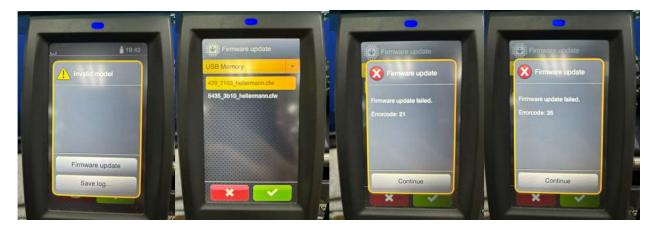
You cannot switch from the CAB firmware to the HellermannTyton firmware. If you encounter this error, the CPU must be replaced.
